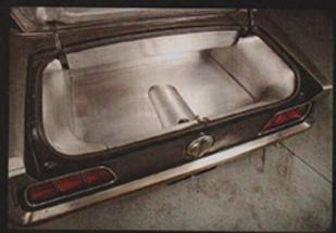
■ The trunk tins do more than look pretty, they conceal the tank, which mounts higher than stock due to the rear roll pan/exhaust design. The air tanks live in the quanter canels, and two Air Zenith pumps mount in the tail panel.
