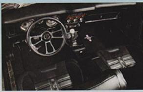
The dash remains almost entirely stock. Yess merely relocated some switches under the dash and shaved their original holes. The reshaped floor meant that existing carpet kits vacuidn't work, so Sieve Ottens at Old Iron Customs and Upholstery in Strathmore came up with a kit from plain loop carpet.
