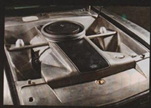
■ The engine cover doubles as the base for the ram air lot. Though really cool, it either hides or steals the thunder from other features like a handmade sespentine system and uncannily smooth inner fender panels and a strut brace. The fenders actually mount from the inner fender panels' lower sides, making the engine compartment that much cleanes.
