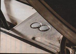
• Lyle Visss made his own pedal assembly to relocate the brake and clutch master cylinders under the cowl. Their reservoirs mount in the cowl, concealed by a custom panel. A pair of handmade hinges and Fox-body Mustang struts support the hood when onen.
